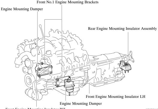
Front Engine Mounting Insulator RH
