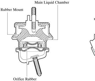
Front Engine Mounting Insulator Cross Section
