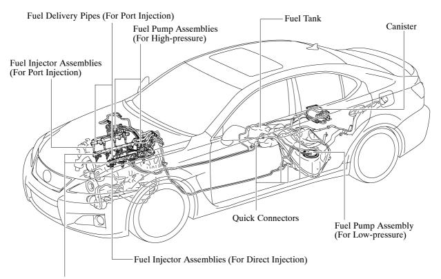
Fuel Delivery Pipes (For Direct Injection)
