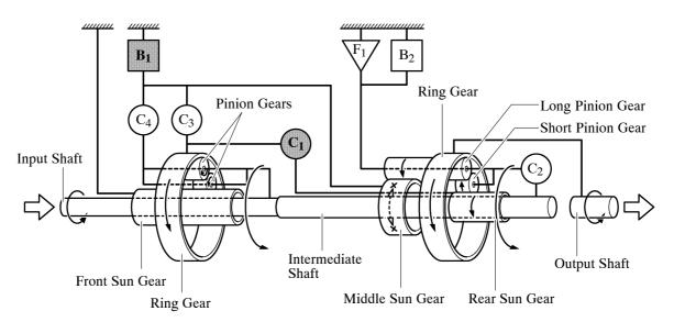
**Front Planetary Gear**
