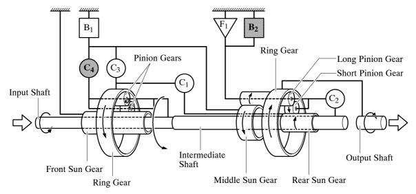
Front Planetary Gear
