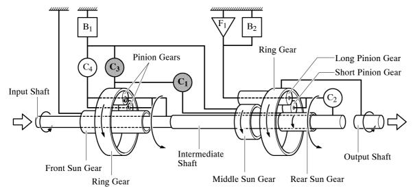
Front Planetary Gear
