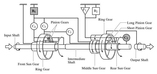
Front Planetary Gear
