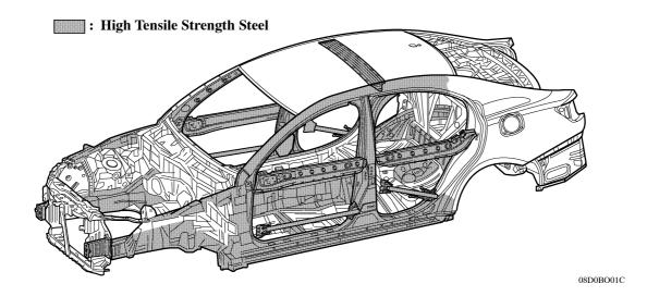
• A brace is installed between the front attachment area of the rear suspension member and the front floor reinforcement, maintaining torsional rigidity. By connecting the braces with a pipe brace, the tendency of the tunnel in the floor to flex is reduced, thus enhancing transverse rigidity.
