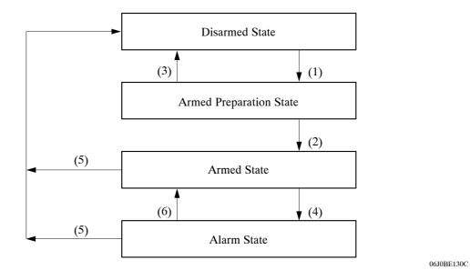
The theft deterrent system activates as described in the diagram below when one of items in the chart occurs in order to cause the system to enter the respective state.
