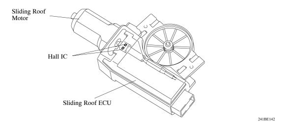
• To control the jam protection function, the sliding roof ECU monitors the amount of movement and judges jamming of the moon roof based on the pulse signals from the Hall IC1, and the moving direction of the moon roof from the phase difference between the pulses from Hall IC1 and Hall IC2.
