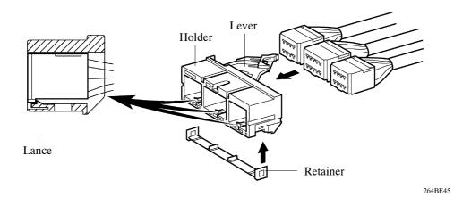
When connecting the holder and connectors to the center airbag sensor assembly, the lever is pushed into position end by rotating it around the axis of the connector lock pin in order to lock the holder securely.
