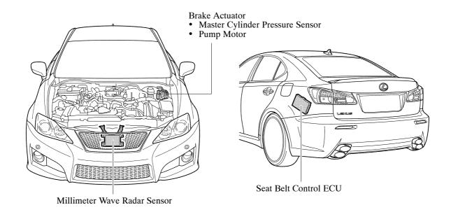
Multi-information Display Master Warning Light PCS Warning Light Network Gateway ECU Main Body ECU RH -(Cowl Side Junction Block RH) Skid Control ECU Assembly Skid Control Buzzer Assembly Yawrate Sensor Steering Sensor Distance Control ECU Assembly Satellite Switch DLC3 Front Seat Outer Belt Front Seat Outer Belt Seat Belt Motor · Seat Belt Motor Front Seat Inner Belt -Front Seat Inner Belt Center Airbag • Seat Belt Buckle Switch • Seat Belt Buckle Switch Sensor Assembly
