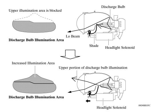
This function is activated by the multiplex network body ECU (front controller). The multiplex network body ECU (front controller) receives a Hi beam turn on signal from the main body ECU RH (cowl side junction block RH) and activates the headlight solenoid built into the headlight unit to slide the shade down.
