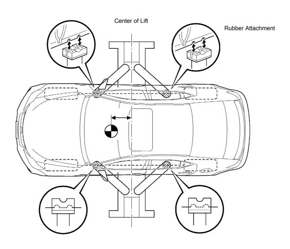
: VEHICLE CENTER OF GRAVITY (Unloaded Condition)
