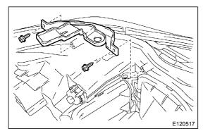
(2) Install the headlight protector retainer with the screw.
