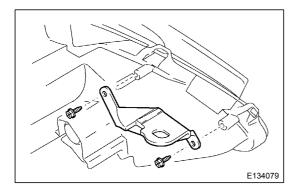
(2) Install the headlight protector retainer with the screw.
