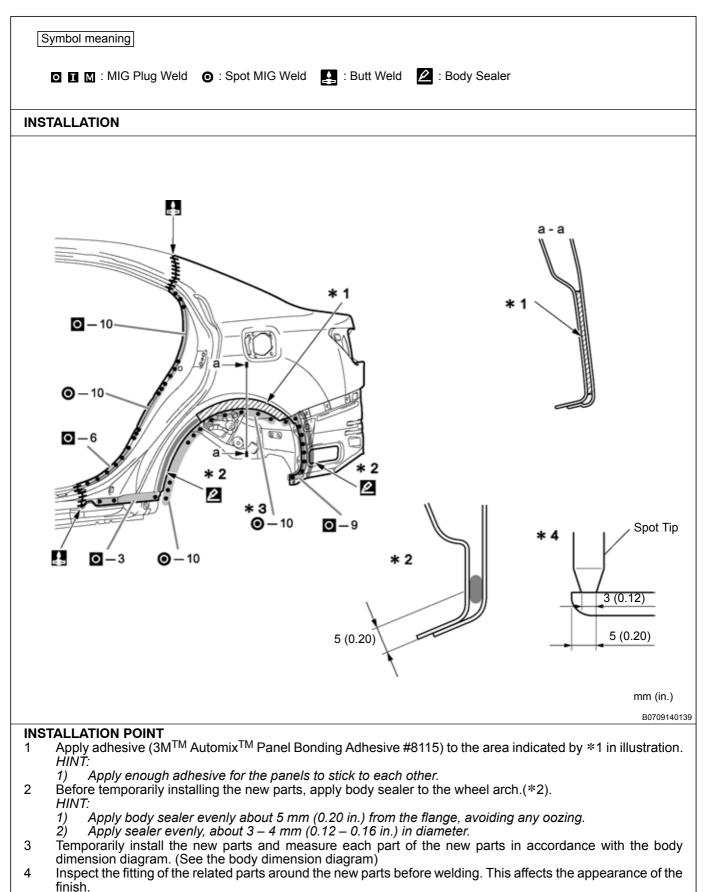
5 Perform spot-welding on the flange indicated by \*3 in the illustration. Modify/cut the spot tip as shown in the illustration (\*4) so that it can fit in to the narrow flange.
