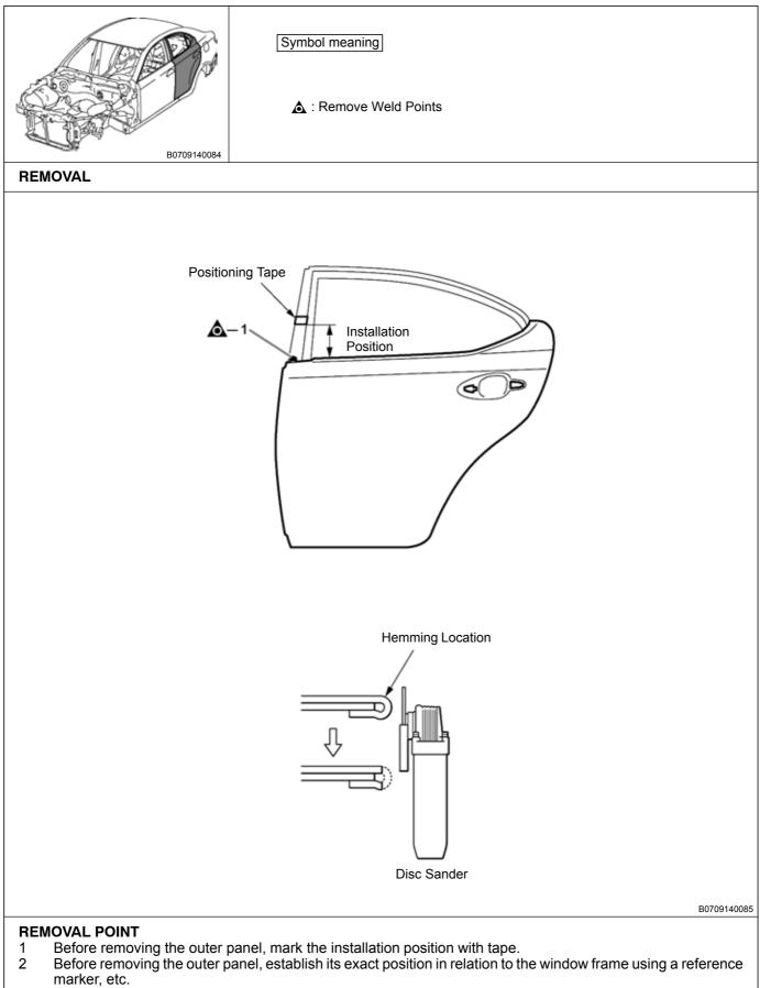
3 After grinding off the hemming location, remove the outer panel.
