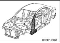
With the front body pillar lower gusset and cowl top side panel removed.
