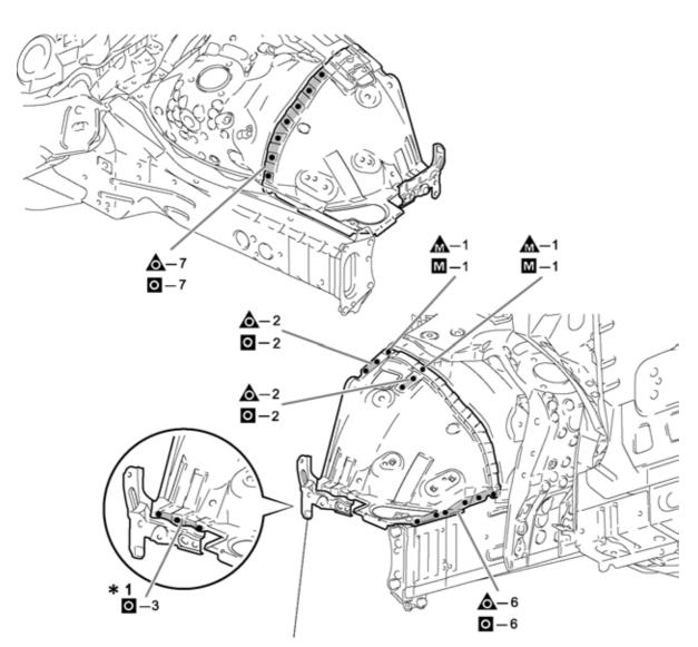
LH: Front End Panel Mounting LH Bracket RH: Radiator Support To Front Fender Bracket
