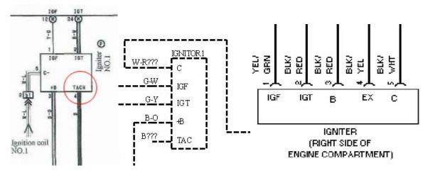
Above are excerpts from three diagrams, each shows the igniter who's plug carrys the tach signal. You can just swap the igniters around on the plugs, in effect there are two tach signals one from each igniter. This is a good example of why the Lextreme diagrams are kinda crap. See the lack of pin numbers in them.
