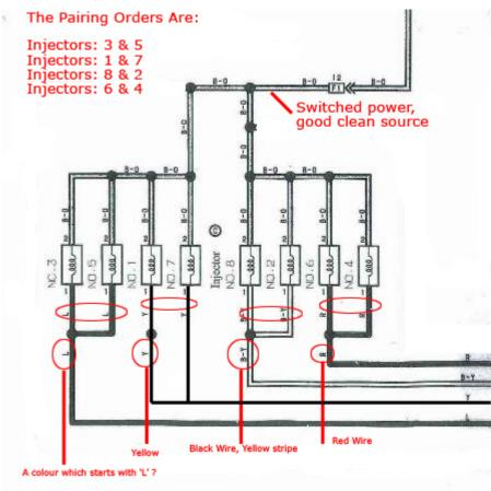
Note the sharing of the cables for the ecu side. The splice is FAR up the loom, if you planning on running sequential injection later move the splice down to very near the ecu when your wiring the engine up.
