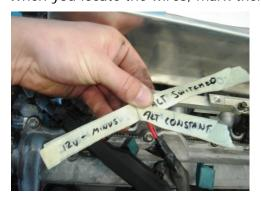
Usually the Alternator plug is FUBAR. It's often brittle, very brittle. Usually broken in someway, or easy to break. If you can leave it on and leave it alone ... do that. Extend the wires as soon as you have a chance and bundle them up in a coil for later use (marked using masking tape at the end of the wires which you will later be connecting. Match the cable types, what I mean is dont put a tiny little gauge extension cable on
