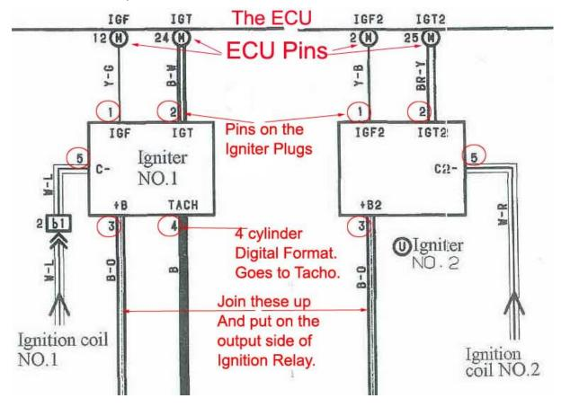
This all seems pretty simple to wire up, it is. The plugs are interchangeable on the igniters, so no1 igniter plug can go on number two and vice/versa. Key Point: you must earth the case of both igniters'. Below is the factory 20v Silver top (cira 1991) igniter and coil mounting which includes the starter relay.
