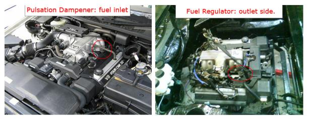
Pulsation Dampener. (it evens out the fuel pulses from the pump, it does NOT impede fuel delivery, or power output (to a point), once your making 300kw's+ you might as well ditch this thing.
