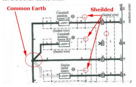
The engine speed sensor is the crank shaft sensor. It travels around in a shielded wire which is basically two wires in a flexible woven wire casing then covered in a plastic casing. The shielding is to protect the signals from interface and at the ECU end needs to be earthed, you can basically collect all the shielded wire up and earth the lot in one go.
