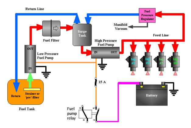
If you use a high pressure 'lift pump' then the fuel will hit the surge tank, find it to be full from the high volume lift pump, and back pressure will form behind the main pump, this pressure will then flow back into the fuel tank via the surge tank's relief line.
