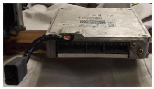
This ecu, if you find it, will never through a code for not having the automatic attached, that plug is a factory fitting. Below is a top image for the same ecu.
