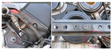
The Crankshaft sensor wiring travels down past passengers side plastic cover, stops at the coil and then continues onward down to the lower pulley. In there is the sensor it's self and a small toothed wheel.
