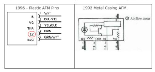
Pay attention to the different configurations of the two Air sensing devices on the 1UZ-FE engine. It's easy to look at the wrong diagram and be thinking you've made a mistake or feel confused.
