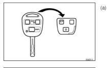
Removing wire-less and immobiliser module from original master key.
