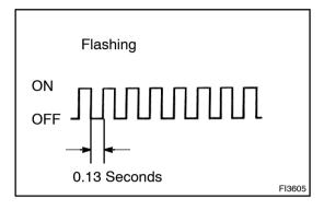
(6) Switch the LEXUS hand-held tester from the normal mode to the check mode. (Check that the MIL flashes.)
