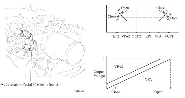
**Accelerator Pedal Depressed Angle**
