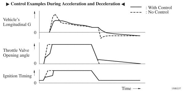
In situations in which low-µ surface conditions can be anticipated, such as when driving in the snow, the throttle valve can be controlled to help vehicle stability while driving over the slippery surface. This is accomplished by turning ON the SNOW switch, which, in response to the amount of the accelerator pedal effort that is applied, reduces the engine output from that of the normal driving level.
