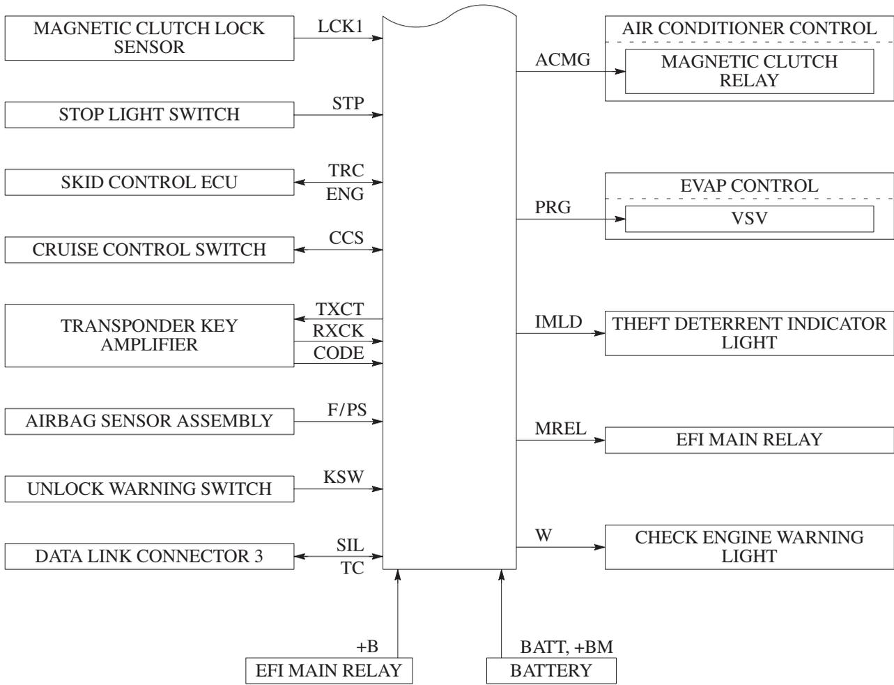
3. Engine Control System Diagram
