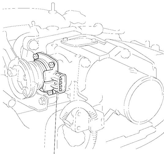
Accelerator Pedal Position Sensor
