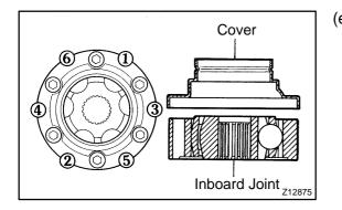
(e) Using a plastic hammer, tap the rim of the inboard joint cover into place. Do this in the order shown, and repeat several times.
