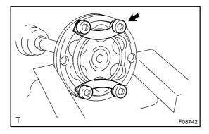
(b) Using bolts, nuts and washers, keep the inboard joint assembly not to take apart.
