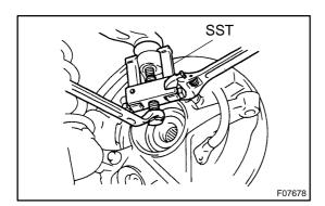
(b) Using SST, disconnect the upper suspension arm. SST 09628-6201 1
