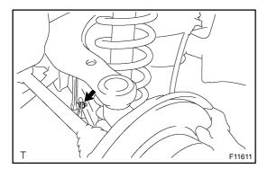
3. **DISCONNECT HEIGHT CONTROL SENSOR LINK**Remove the nut and disconnect the height control sensor link from lower arm bracket.
