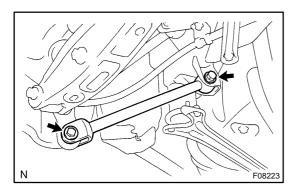
**4. REMOVE NO. 1 LOWER SUSPENSION ARM** Remove the 2 bolts, nuts, and No. 1 lower suspension arm.
