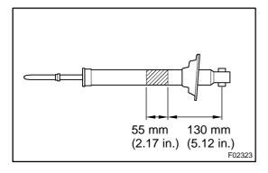
2. DRILL HOLE TO DISCHARGE GAS FROM CYLINDER Using a drill, make a hole in the cylinder as shown to discharge the gas inside.
