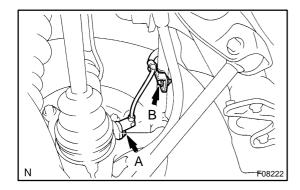
20. CONNECT RH AND LH ABS SPEED SENSORS AND WIRE HARNESS
