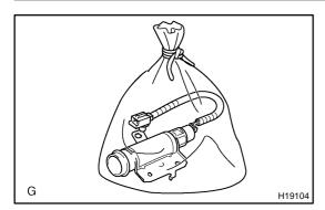
3. DEPLOYMENT WHEN DISPOSING OF SIDE AIRBAG ASSEMBLY WITH AIRBAG DEPLOYED IN COLLISION
