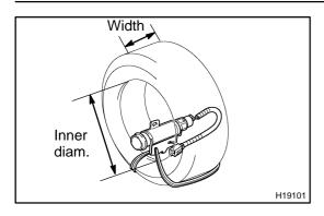
Position the curtain shield airbag assembly inside the tire with the airbag deployment direction facing inside.
