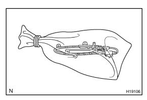
e) Put the removed curtain shield airbag assembly into a clear plastic bag and keep it in a safe place.
