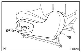
Power adjuster type: INSTALL FRONT SEAT CUSHION SHIELD
