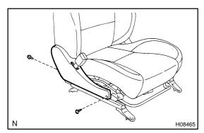
4. Manual adjuster type: INSTALL FRONT SEAT CUSHION INNER SHIELD Install the front seat cushion inner shield with the 2 screws.
