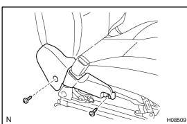
3. Power adjuster type: INSTALL FRONT SEAT CUSHION INNER SHIELD Install the front seat cushion inner shield with the 2 screws.
