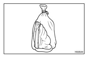
(g) Dispose of the side airbag assembly.
