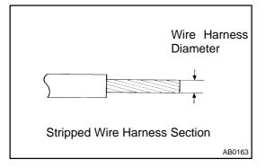
(b) Using a service-purpose wire harness, tie down the side airbag assembly.
