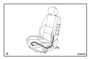
(b) Disconnect the side airbag assembly connector.
