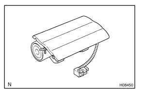
(a) Remove the front passenger airbag assembly (See page RS-28 ).
