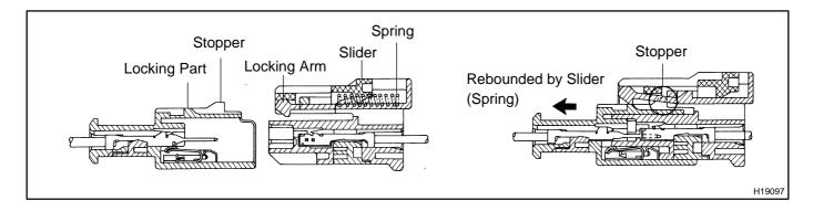
(5) Connector twin-lock mechanism:
