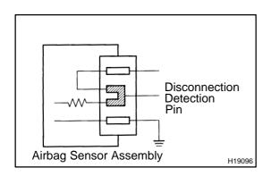
(3) Electrical connection check mechanism:
