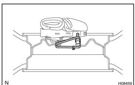
Using 3 wire harness, wind the wire harness at least2 times each around the bolts installed on the leftand right sides of the steering wheel pad.
