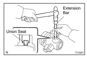
(b) Using a plastic hammer and extension bar, lightly tap in a new union seat.
