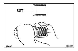
(e) Carefully slide the tapered end of SST over the teflon rings until they fit to the control valve assembly.
