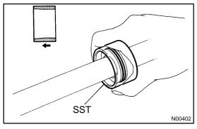
(f) Carefully slide the tapered end of SST over the teflon ring until it fits to the steering rack.
