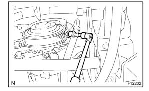
(b) Connect the pressure feed tube with the union bolt.
