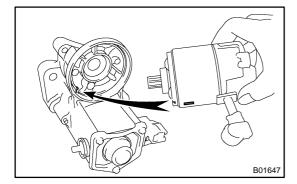
(c) Pull out the field frame together with the armature. HINT:
