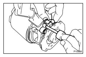
(c) Using a screwdriver, hold the spring back and disconnect the brush from the brush holder. Disconnect the 4 brushes, and remove the brush holder.
