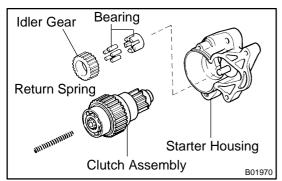
(b) Remove the starter housing, idler gear, bearing, clutch assembly and return spring from the magnetic switch.
