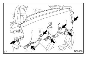
(j) Remove the 5 bolts, 2 nuts, air intake chamber and 2 gaskets
