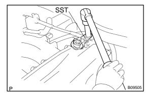
(b) Using SST, tighten the pulsation damper. SST 09612-24014 (09617-24011)
