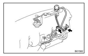
(c) Install the bolt holding the fuel inlet pipe to the intake manifold.
