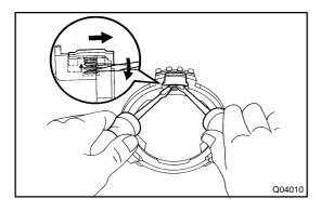
(e) Remove the 3 shifting keys and key springs by carefully levering up the shifting key spring with one screwdriver and levering the shifting key away from the reverse synchronizer ring with another screwdriver.
