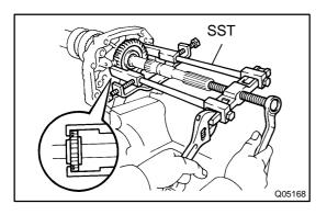
(b) Using SST, remove the reverse gear. SST 09950-40011 (09951-04020.
