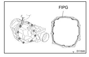
(b) Remove the 9 bolts and wire harness clamp from the extension housing.
