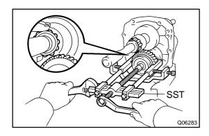
(b) Using SST, remove the rear bearing, spacer, counter 5th gear and bearing.
