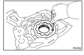
(c) Inspect the rotor for the body clearance.
