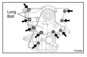
(c) Apply seal packing to the oil pump as shown in the illustration.
