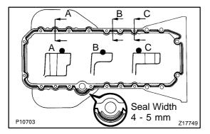
(c) Apply seal packing to the No. 1 oil pan as shown in the illustration.
