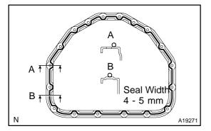
(b) Apply seal packing to the No. 2 oil pan as shown in the illustration.
