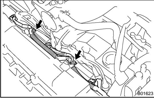
**5. REMOVE IGNITION COILS AND HIGH-TENSION CORDS SET ASSEMBLY**
