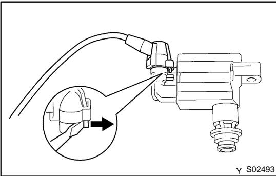
**6. REMOVE IGNITION COILS FROM HIGH-TENSION CORD SET**
