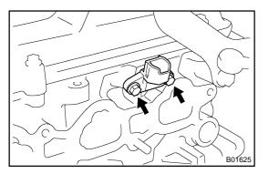
11. REMOVE CAMSHAFT POSITION SENSOR
