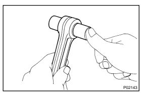
(e) Check the piston pin fit at room temperature. Coat the piston pin with engine oil and push it into the connecting rod with your thumb.
