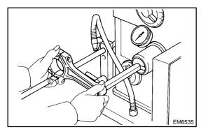
(d) Using a pin hole grinder, bore the bushing to obtain the standard specified clearance (See page EM-87) between the bushing and piston pin.
