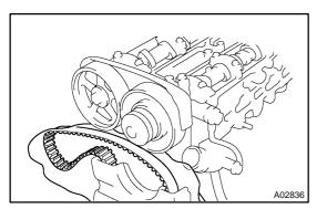
25. DISCONNECT TIMING BELT FROM CAMSHAFT TIM-ING PULLEYS (See page EM-17)
