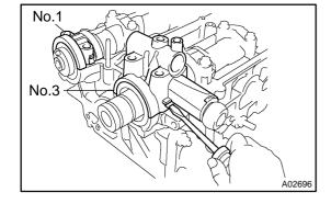
(c) Using a screwdriver, pry out the Nos. 1, 3 camshaft bearing caps and oil seals.
