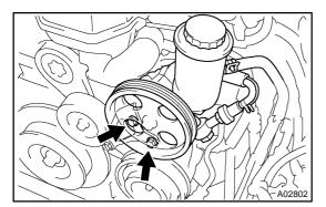
(d) Remove the 2 bolts, and disconnect the vane pump from the pump bracket.
