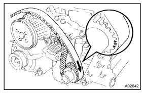
(c) Install the timing belt on the crankshaft timing pulley and idler pulley.
