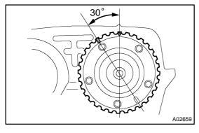
(b) Check that the outer circumference of the VVT-i pulley easily rotates through 30°.
