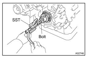
(b) Remove the crankshaft timing pulley.
