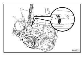
(b) Using a timing light, check the ignition timing.Ignition timing:10 ± 2° BTDC @ idle
