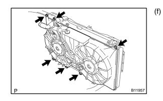
Remove the 6 bolts and electric cooling fan.
